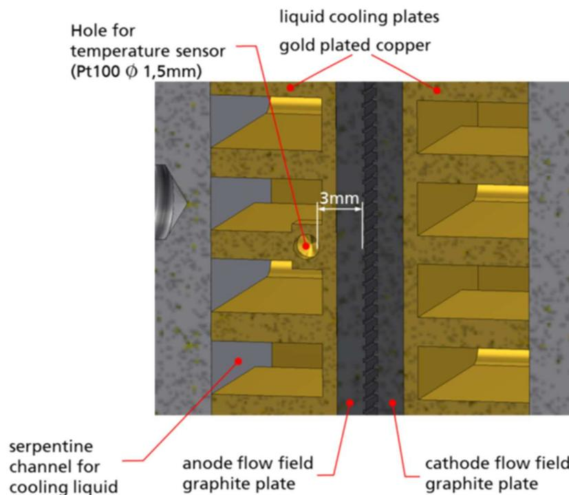
Figure 7: Liquid cooling of Baltic cell unit
