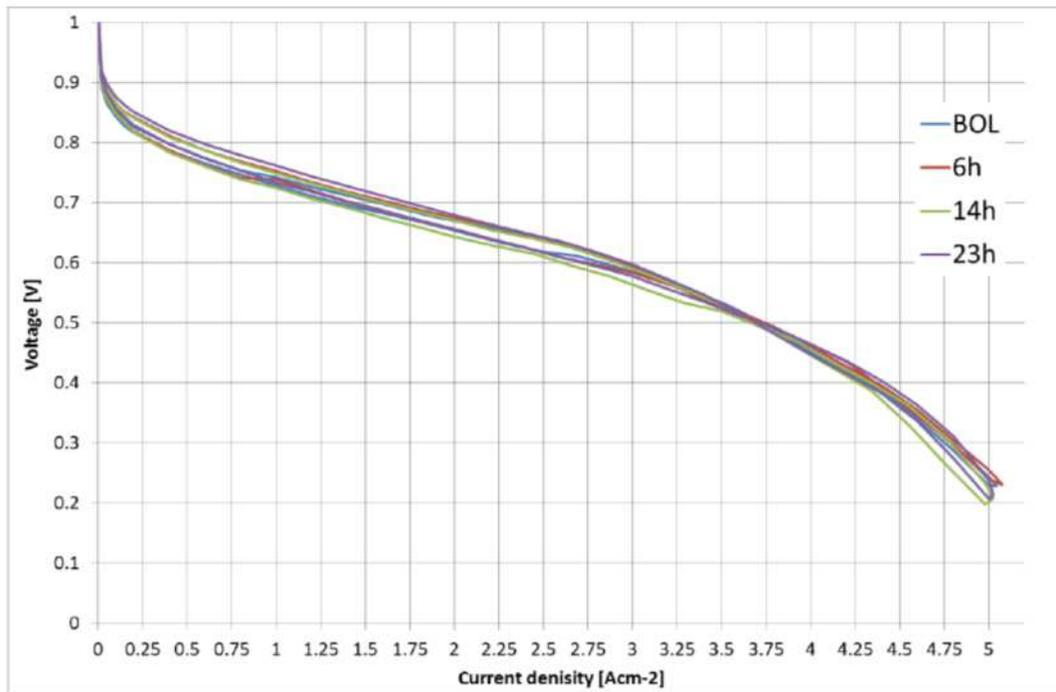
Figure 2: Reproducibility of JRC test cell: Test results of JRC with one MEA.
