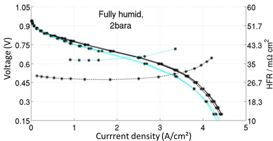
Figure 9: Reproducibility with baltic test cell hardware by using 1 MEA for several tests. Measurements of Fraunhofer ISE
