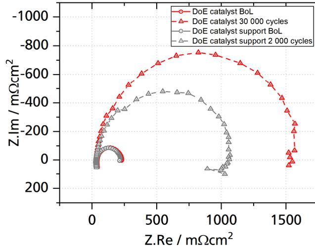
Figure 13: Polarization curve and EIS in conditions CatOutCold.
