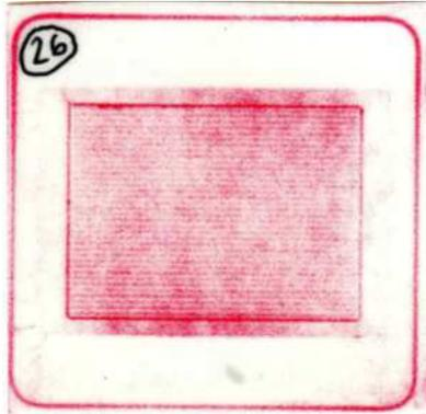
Figure 6: Even compression of the active cell area tested with pressure paper
