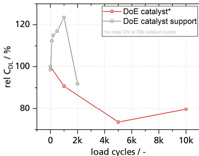
Figure 20: Relative losses in Double Layer Capacity during ASTs.
