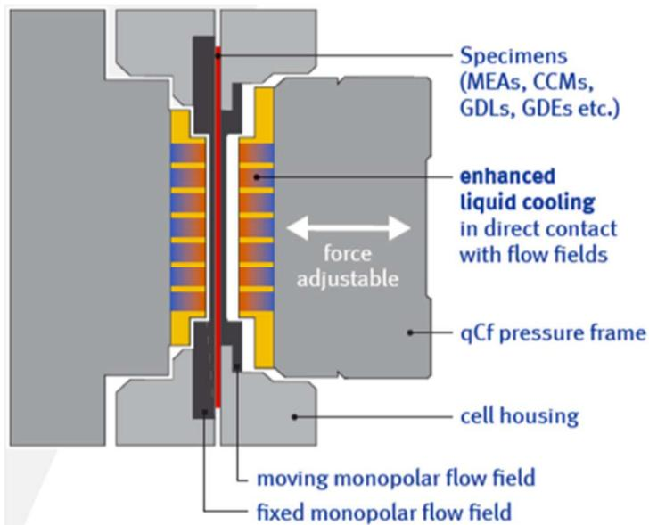
Figure 5: Design of Baltic cell unit
