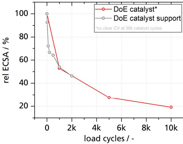
Figure 19: Relative losses in ECSA during ASTs.
