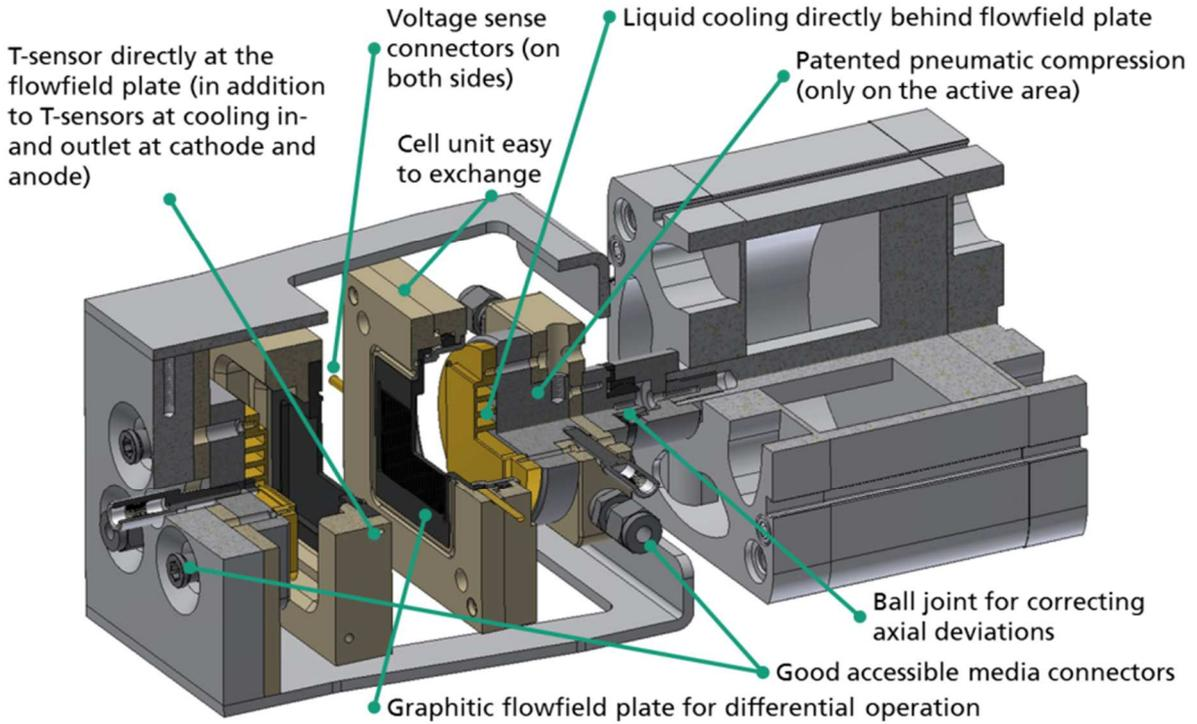
Figure 4: Design of Baltic test cell hardware
