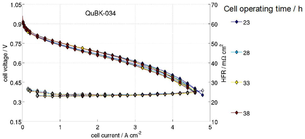
Figure 22: Comparison of polarization curves. Testing was done at Fraunhofer ISE for Baltic hardware.
