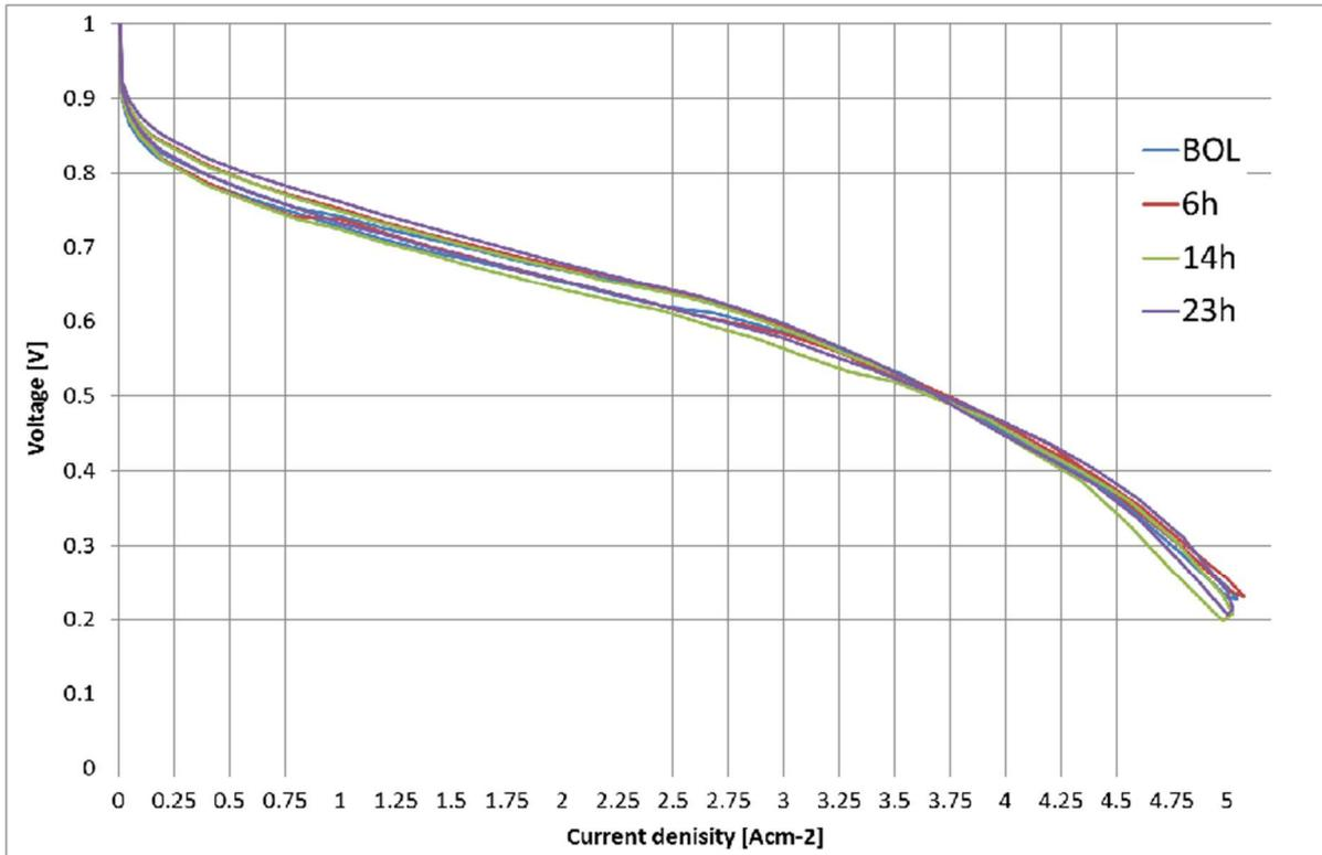
Figure 21: Comparison of polarization curves. Testing was done at JRC for JRC test cell hardware.
