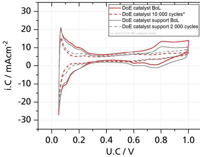
Figure 17: Cyclovoltammety BoL and EoT.
