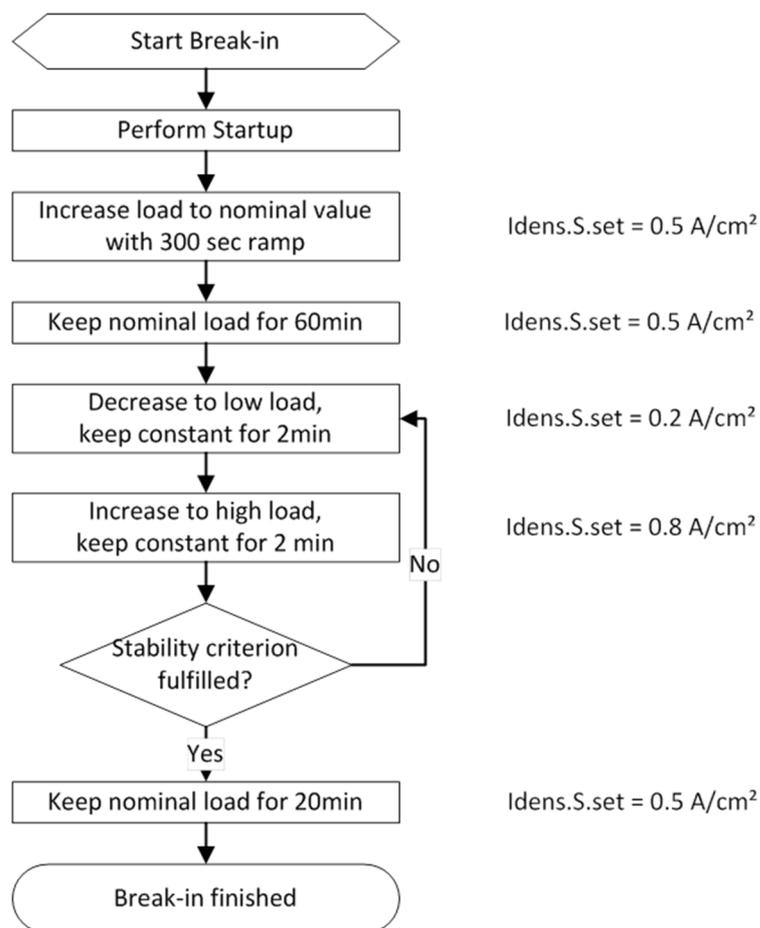
Figure 10: General break-in procedure as defined by the STACK-TEST project, figure reproduced from the STACK-TEST master document (<http://stacktest.zsw-bw.de>)
